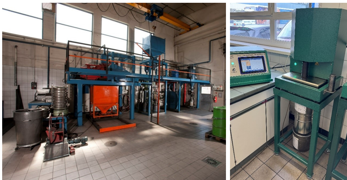
Figure 1. Left: Dry aggregate preparation at the R&D Carbon research center, Right: RDC-194 ramming behavior equipment used for temperature window testing.
